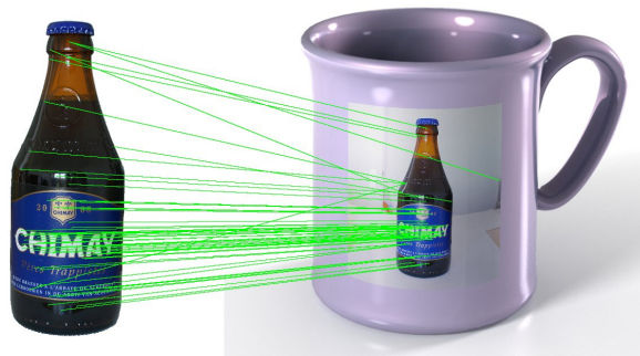
Figure 7: The detected interest points of the left image are matched with the detected interest points of the right image. Unfortunately, the left image is a bottle and the right image is a mug with an image of the same bottle on it. Interest point detectors that use only 2-dimensional information are not able to detect this difference, which is important for a robot in a human living environment. Image source: [18]
